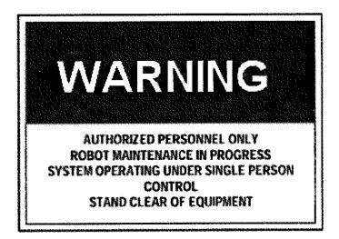
Figure 6-15 - Sample Warning Sign Used During Robot Maintenance
