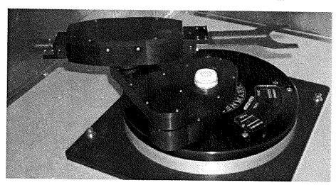
Figure 6-19 - Leveling the Genmark Robot Lower Arm
